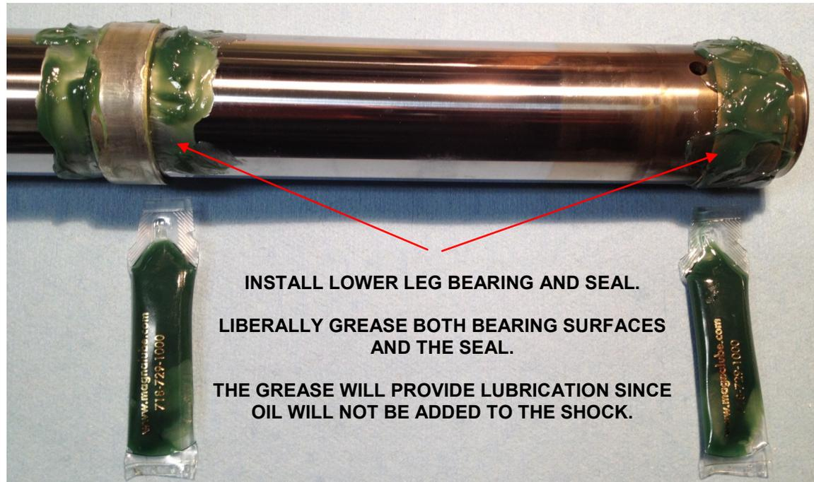
**INSTALL LOWER LEG BEARING AND SEAL.
